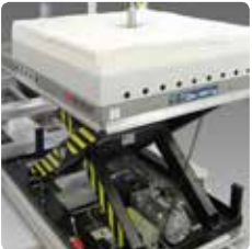
Replacement floor, adjustable in height
