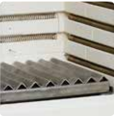
Integrated collecting drawer for moulding material
