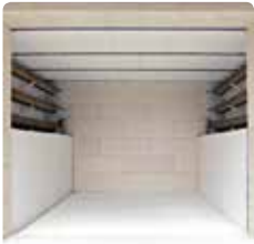
SiC cover for heating elements
