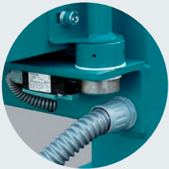
Security switch mounted in protected position
