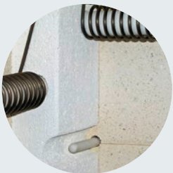
Thermocouple mounted in protected position
