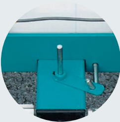
Air supply slide operated from front, improved air supply handling
